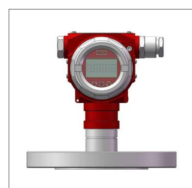
Safety is the primary concern of food and pharmaceutical production. Sanitary pressure transmitter specifically designed for the food and pharmaceutical industry, adopts stainless steel external structure. And the wetted parts with superb stainless steel 316L diaphragm and complete welding technology, the polished finish ≤0.4 u. Hygienic filling liquids in line with FDA standard. Suitable for CIP and SIP cleaning. Richen international standard process connection for optional.
