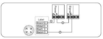
Connect the positive power supply (P+) to the terminal 1/brown wire of pressure transmitter;
