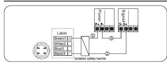
1 Connect the positive power supply (P+) to the terminal 1/brown wire of pressure transmitter;
